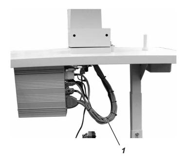
To make the tilting of the machine head possible, make sure that the cables leading from the head through the opening in the table top to either the 15-way multiple pin strip at the control box and to the cable duct are long enough. For this purpose the cables must be laid to form an arc 1 with the help of the cable ties.
