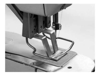
From the factory, the automatic bartacker 511-213 is set for the processing of normal fabrics.
