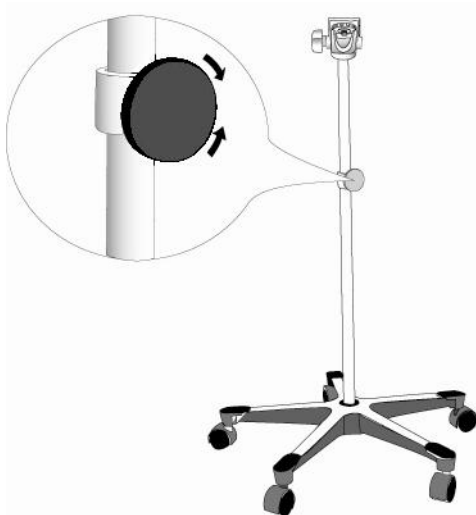
Figure 13. Adjusting the height of the mobile stand.
