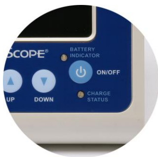
Figure 8. Front panel LEDs indicate battery usage and charge status.
