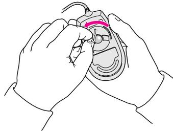
Turn the ring a very short distance. When the recessed area on the ring is lined up with the recessed area surrounding the ring, the mouse is unlocked.
