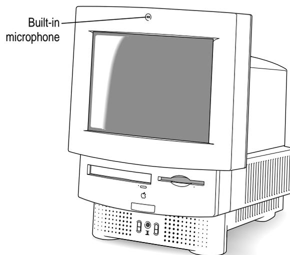
**WARNING** Do not stick any small objects into the built-in microphone. Doing so may damage your equipment.
