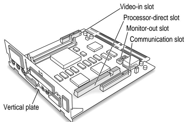
This appendix contains instructions for installing a PDS card or communication card. To install a video input card or an external video connector card, follow the instructions that came with the card.
