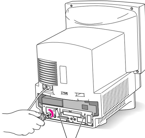
Reinsert both retainer screws into the vertical plate.
