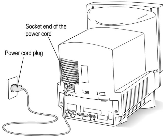
**WARNING** This equipment is intended to be electrically grounded. Your Macintosh is equipped with a three-wire grounding plug—a plug that has a third (grounding) pin. This plug will fit only a grounded AC outlet. This is a safety feature. If you are unable to insert the plug into the outlet, contact a licensed electrician to replace the outlet with a properly grounded outlet. Do not defeat the purpose of the grounding plug!
