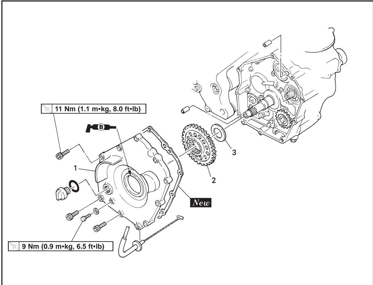
Extend of removal: ① Primary driven gear removal
