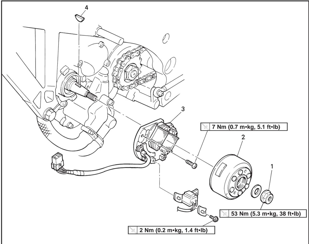
Extend of removal: ① CDI magneto removal
