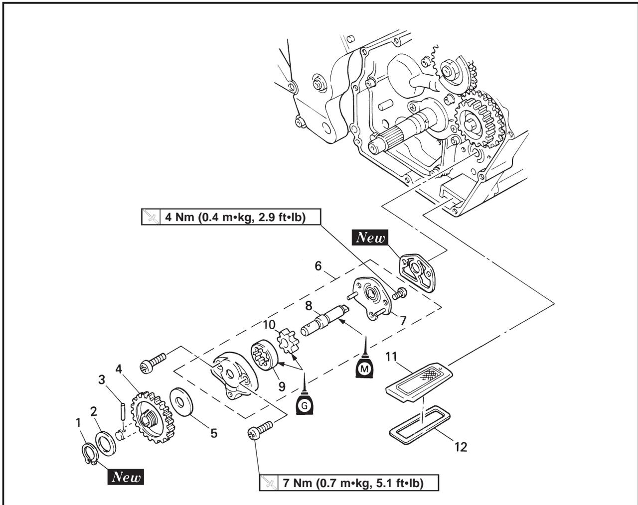
Extend of removal: ① Oil pump removal and disassembly      ② Strainer removal
