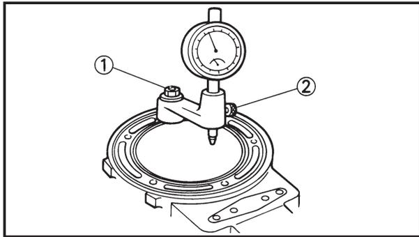
2. Loosen the stand installation bolt ①, then rotate the dial gauge stand and set it close to the center of the piston. Tighten the stand installation bolt again.
