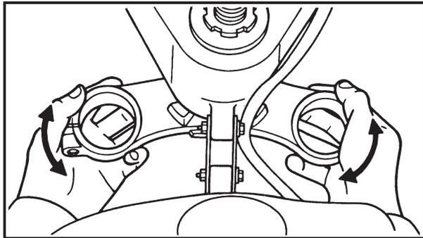
6. Check the steering shaft by turning it lock to lock. If there is any binding, remove the steering shaft assembly and inspect the steering bearings.
