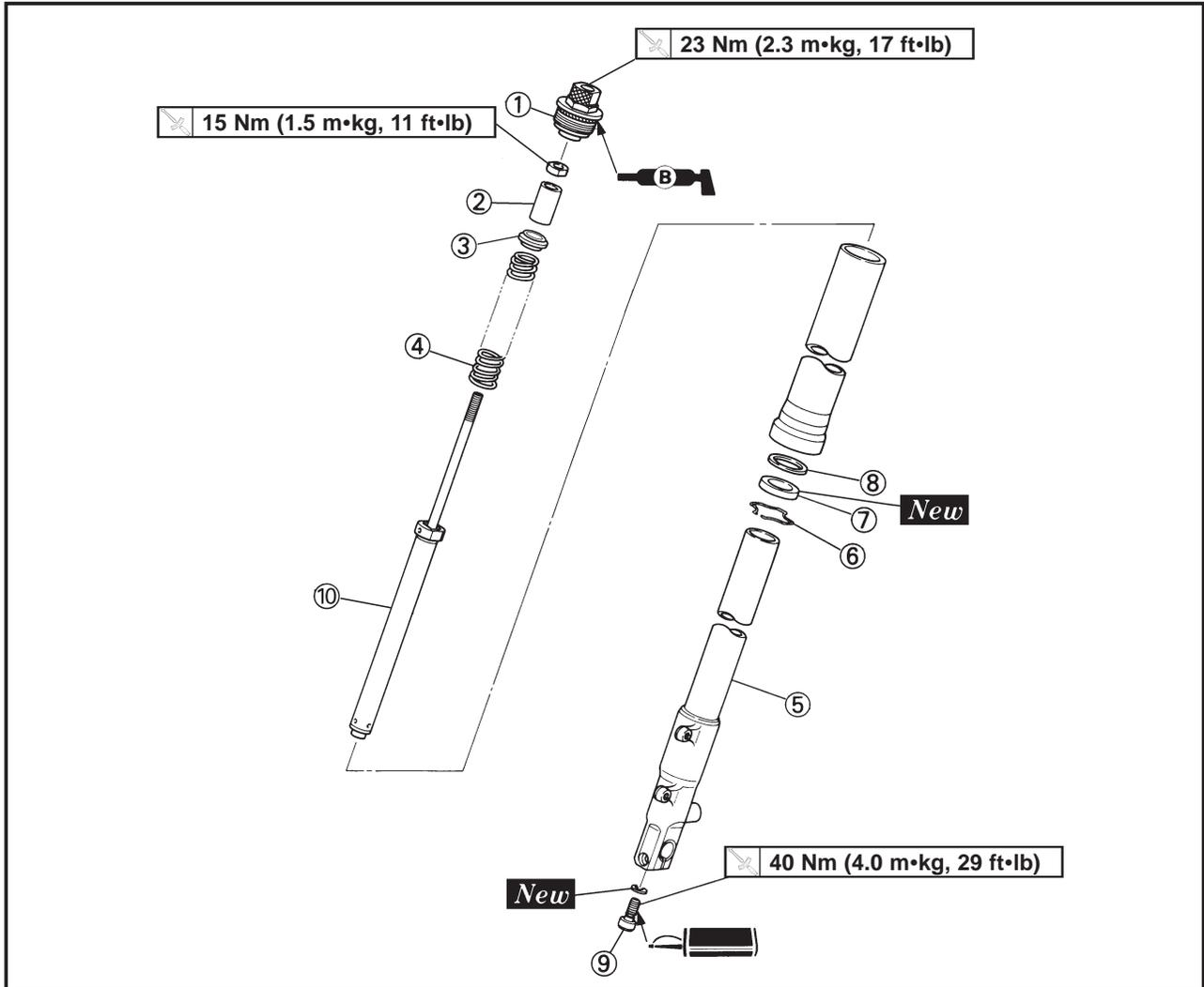
Extend of removal: ① Oil seal removal
