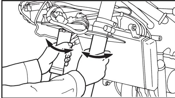
9. After tightening the nut, check the steering for smooth movement. If not, adjust the steering by loosening the ring nut little by little.
