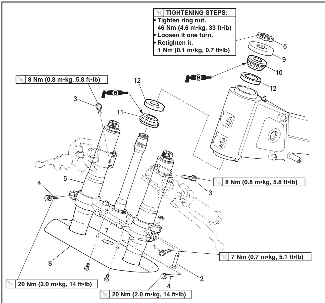
Extend of removal: ① Under bracket removal      ② Bearing removal
