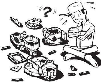
4. During the machine disassembly, clean all parts and place them in trays in the order of disassembly. This will speed up assembly time and help assure that all parts are correctly reinstalled.
