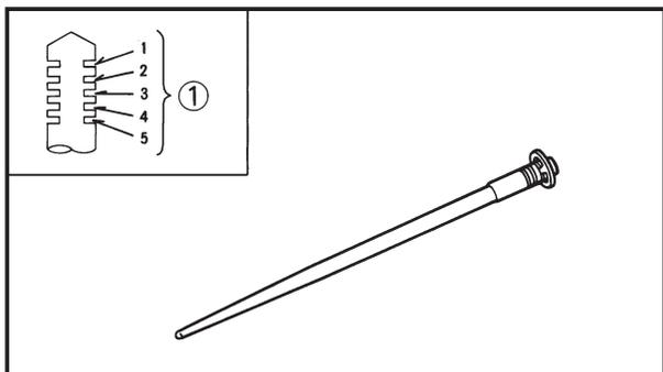
4. Adjustment of jet needle clip position
