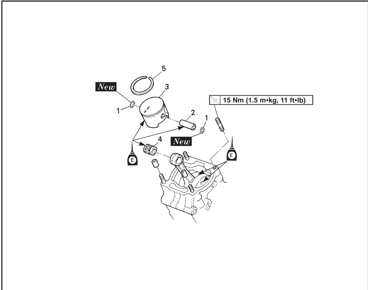
Extend of removal: ① Piston and piston ring removal
