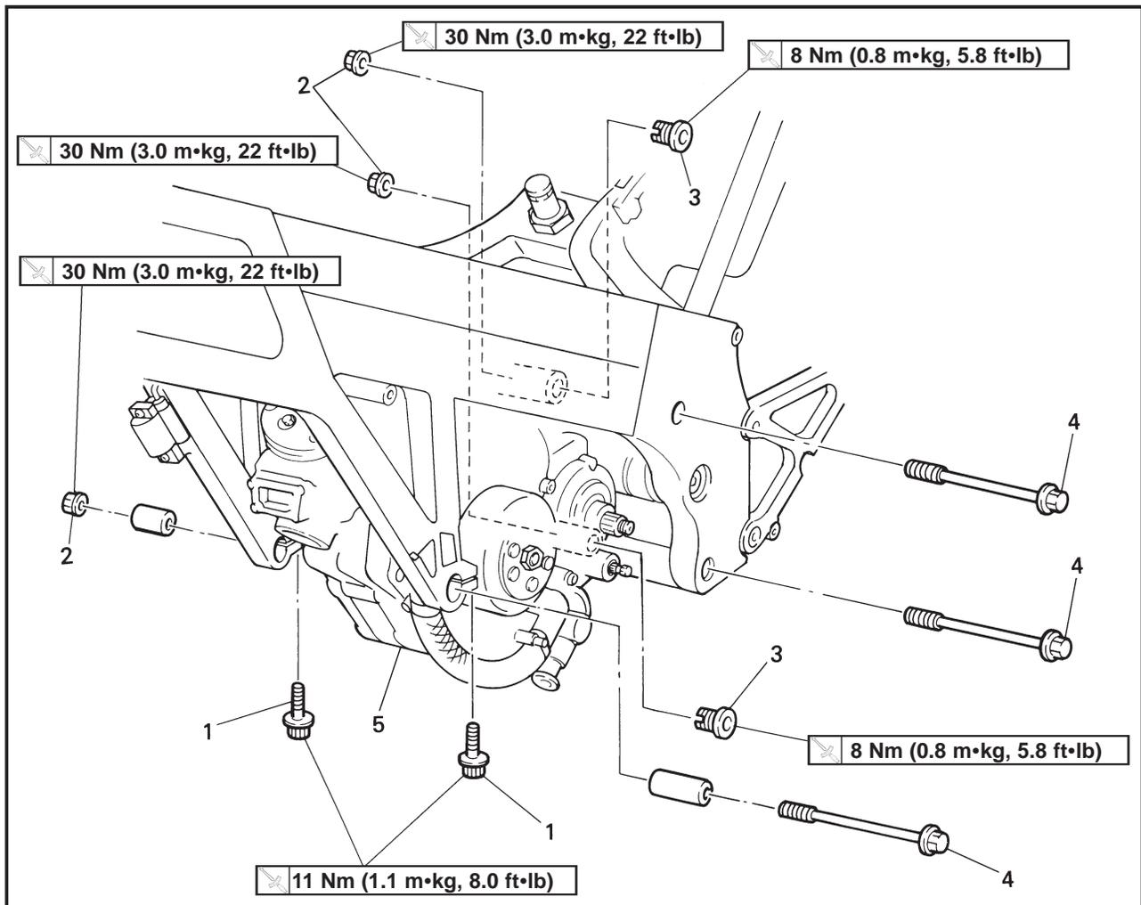
Extend of removal: ① Engine removal
