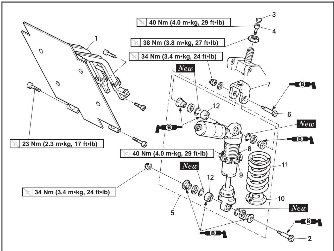
Extend of removal: ① Rear shock absorber removal
