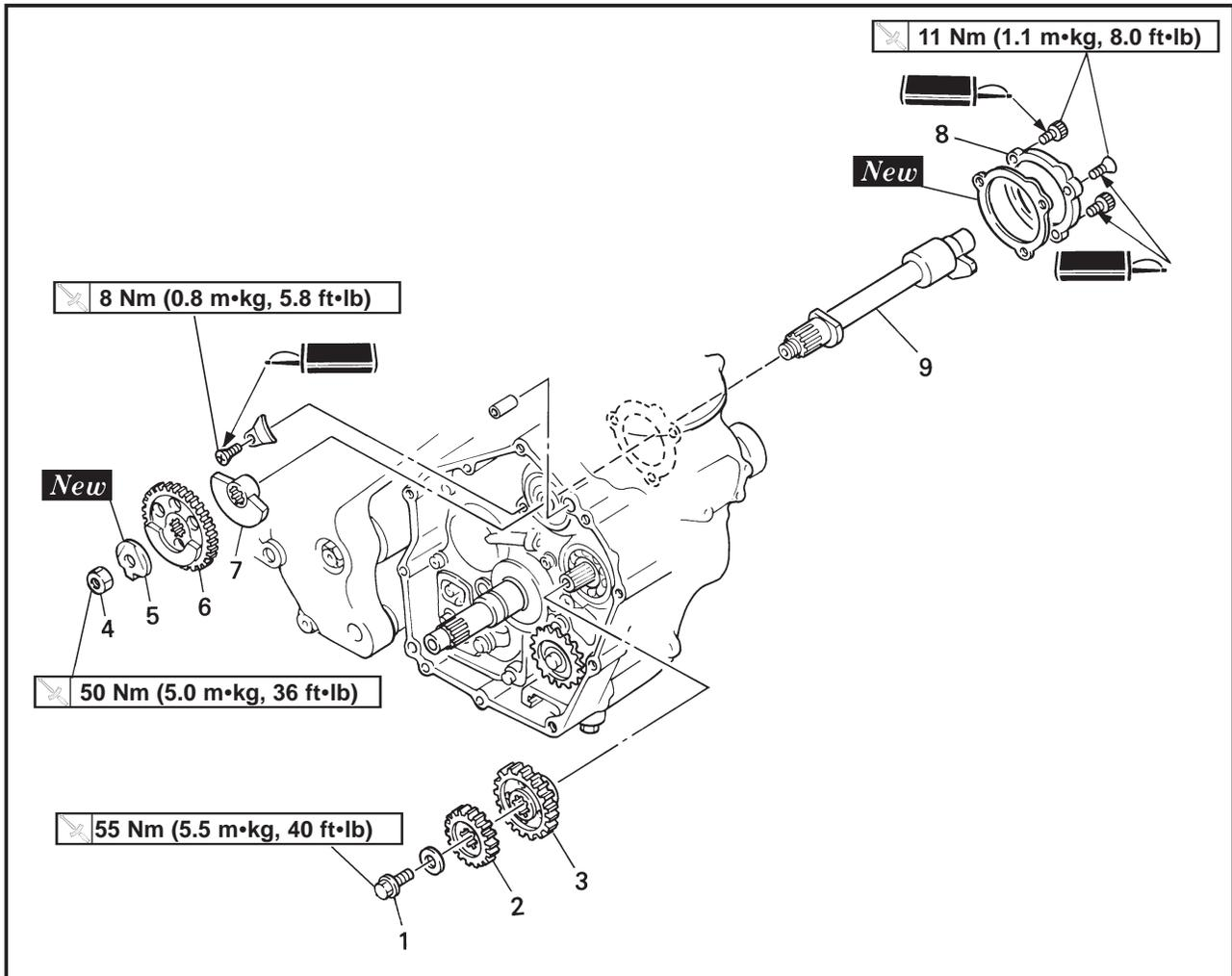
Extend of removal: ① Primary drive gear removal      ② Balancer shaft removal
