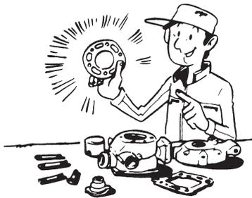
3. When disassembling the machine, keep mated parts together. They include gears, cylinders, pistons, and other mated parts that have been "mated" through normal wear. Mated parts must be reused as an assembly or replaced.
