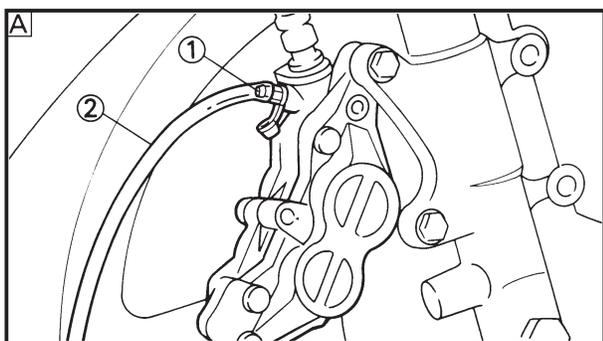
2. Connect the transparent hose ② to the bleed screw ① and place a suitable container under its end.
