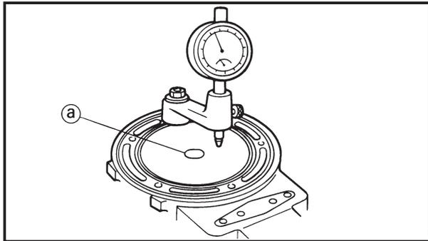
3. Set the piston at top dead center (TDC), then measure the piston protrusion.
