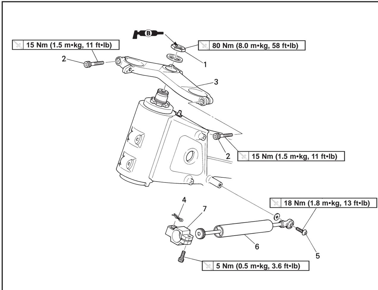
Extend of removal: ① Handle crown removal                      ② Steering damper removal
