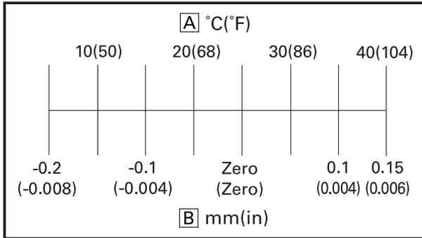
When the cylinder gasket is changed, measure the protruding (or sinking) amount of the piston above (below) the cylinder top and then change the cylinder gasket so that the following approximate relation can be achieved between the temperature and the piston protruding amount. (The table shows an example when the air pressure is 1013 hPa (760 mmHg).)
