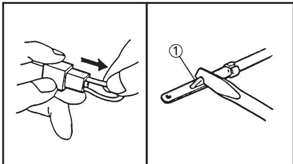
3. Connect and disconnect the connector two or three times.
