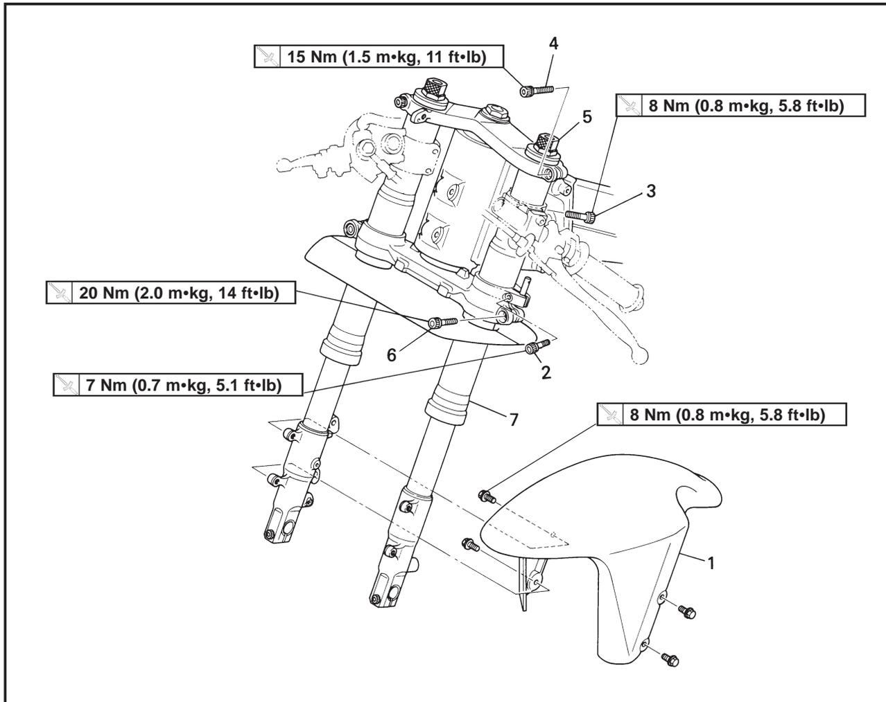
Extend of removal: ① Front fork removal
