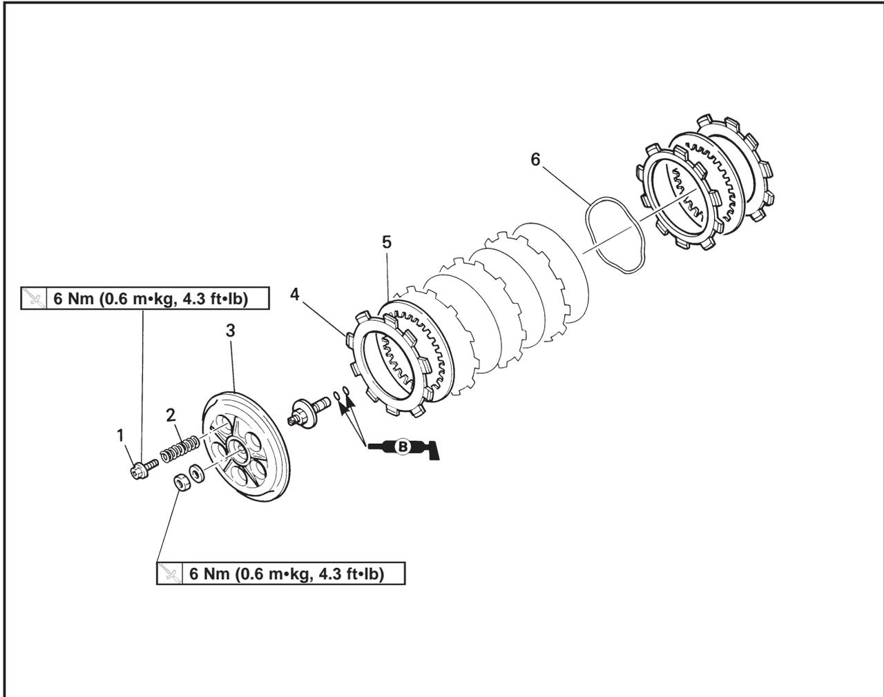
Extend of removal: ① Clutch plate and friction plate removal
