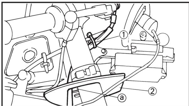
2. Pass the brake hose through the clamp ① and hole ① of the inner fender ②.
