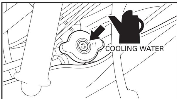
2. The cooling system is filled with coolant at the factory to prevent rusting. Be sure to replace coolant with soft water before riding.
