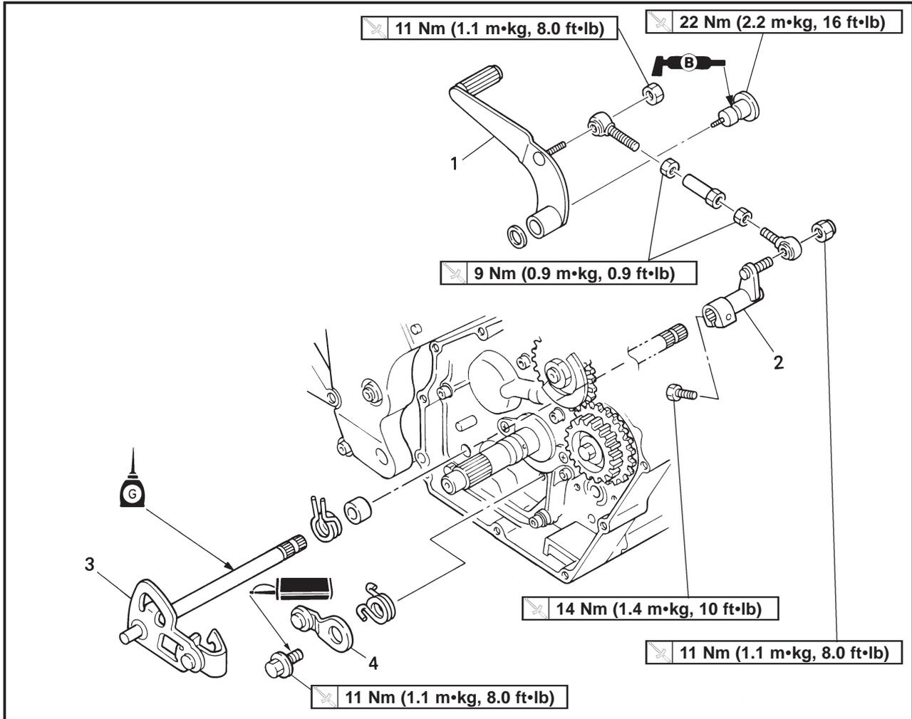
Extend of removal: ① Shift shaft removal      ② Stopper lever removal
