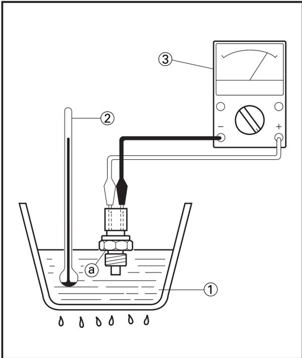
3. Immerse the thermo unit with a tester lead connected in a container containing cooling (tap) water ① down to the upper threaded portion ③.
