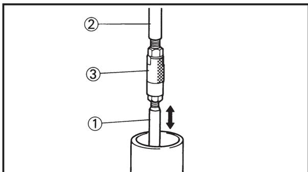
14. After filling, pump the damper rod ① slowly up and down more than 10 times to distribute the fork oil.
