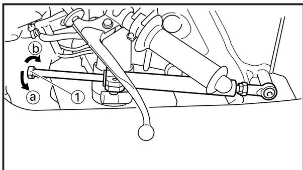
**Stiffer (a) → Increase the compression damping force. (Turn the adjuster ① in.)**
