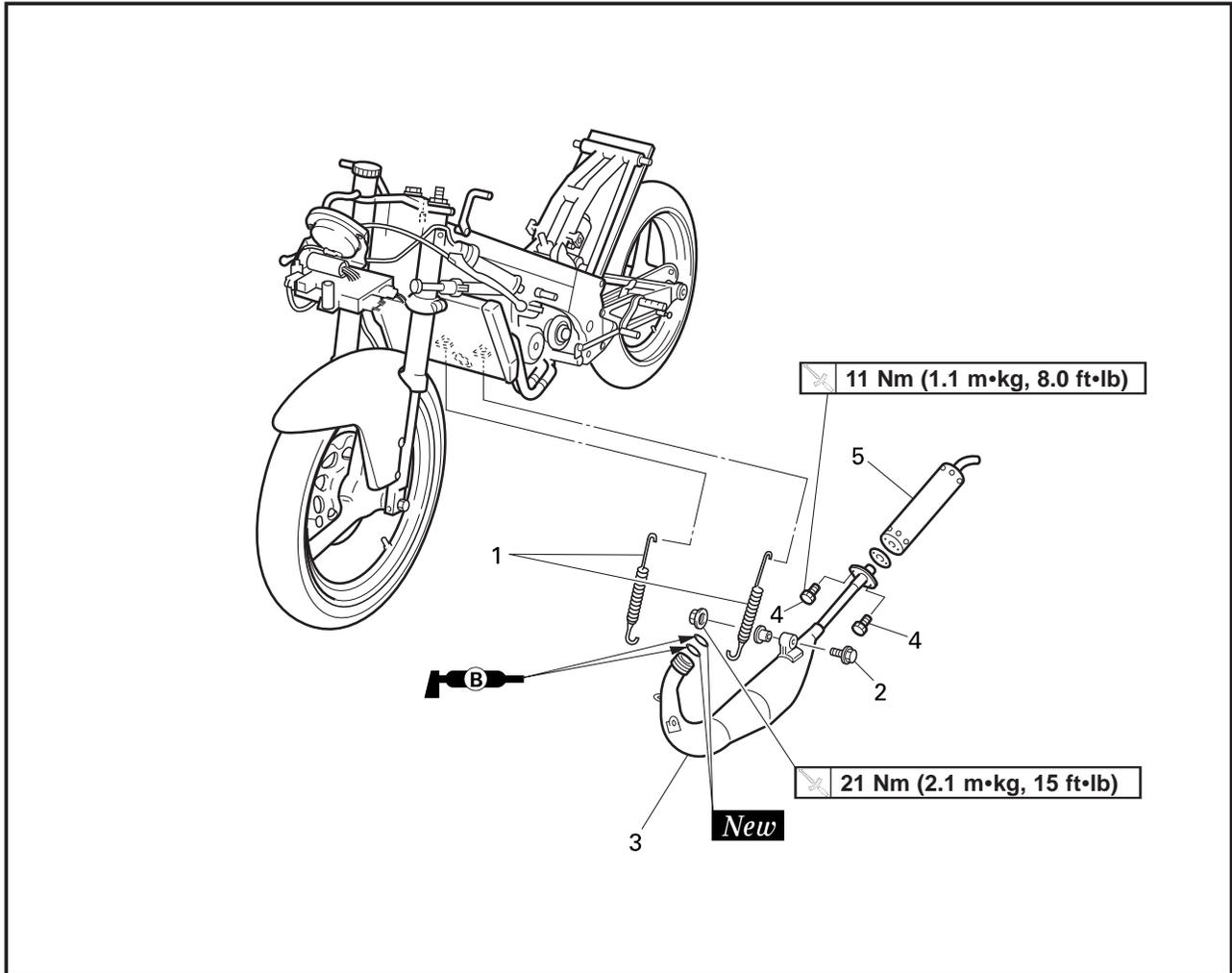
Extend of removal:    ① Exhaust pipe removal                      ② Silencer removal
