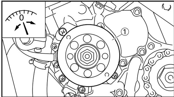
3. Rotate the magneto rotor ① until the piston reaches top dead center (TDC). When this happens, the needle on the dial gauge will stop and reverse directions even though the rotor is being turned in the same direction.
