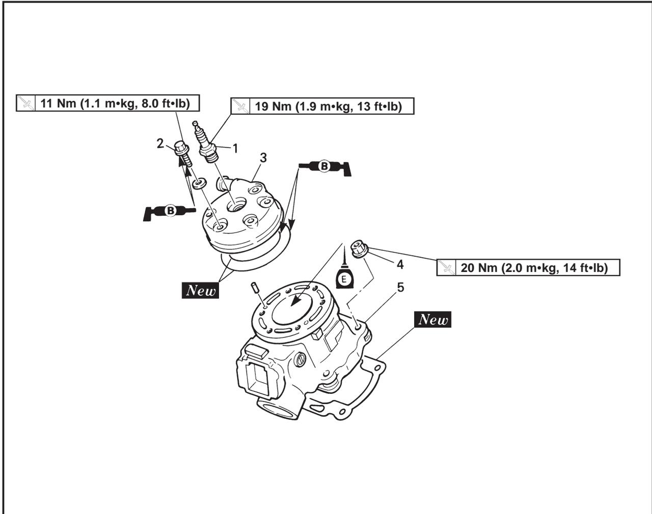
Extend of removal: ① Cylinder head removal      ② Cylinder removal
