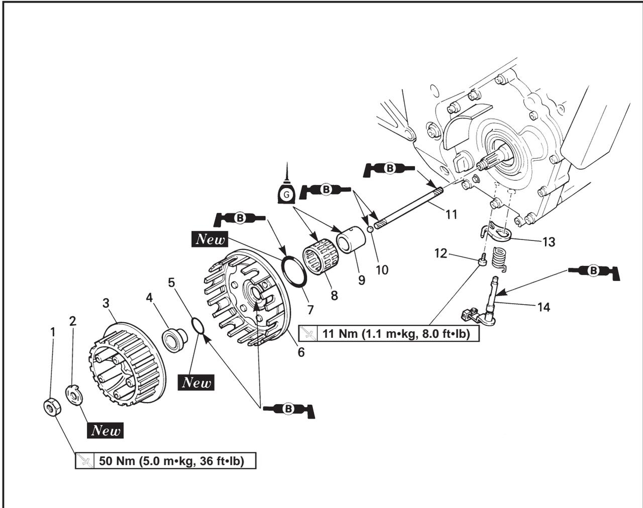
Extend of removal: ① Clutch housing removal
