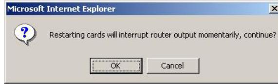
**CAUTION** Clicking the OK button will cause a momentary interruption to video passing through the Routing switcher. Clicking the Cancel button, while not advised, will stop the restart process allowing you to restart the board during a scheduled service time. However, the new software will not be applied until the boards are restarted.
