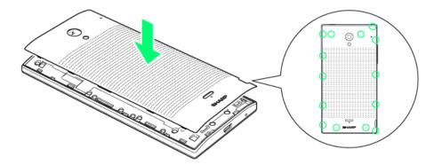
• Press firmly where marked o so there are no gaps. Be careful not to press excessively and damage the battery cover.
