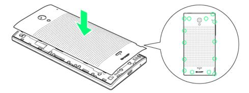
• Press firmly where marked o so there are no gaps. Be careful not to press excessively and damage the battery cover.
