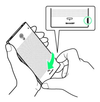
Lift where marked o (indent) and create a gap between the battery cover and the phone.
