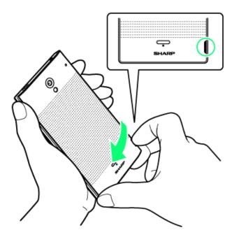
• Lift where marked o (indent) and create a gap between the battery cover and the phone. Continue by sliding your finger completely around the phone under the battery cover to remove.
