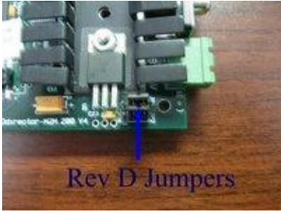
**Rev D: JP1** is the DB37 pin 20 jumper that supplies the VRail output voltage with maximum current of 0.5A. JP1 1-2 connects VRail to Vin (nominally 12VDC), JP1 2-3 connects VRail to +5V.
