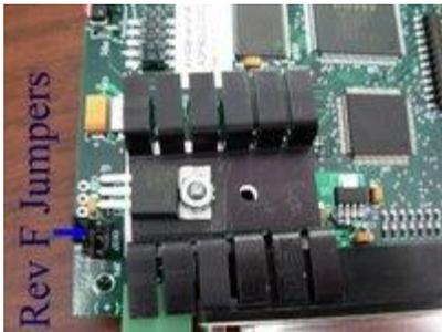
**Rev F: JP1** is the DB37 pin 20 jumper that supplies the VRail output voltage with maximum current of 2A. JP1 1-2 connects VRail to Vin (nominally 12VDC), JP1 2-3 connects VRail to +5V.
