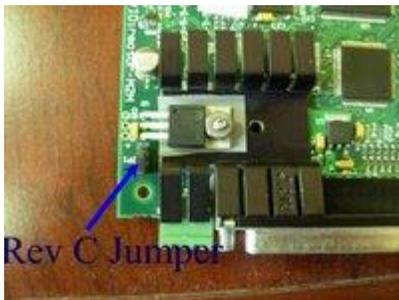
**Rev C:** **JP1** is the DB37 pin 20 jumper that supplies the VRail output voltage with maximum current of 0.5A. JP1 1-2 connects VRail to Vin (nominally 12VDC), JP1 2-3 connects VRail to +5V.
