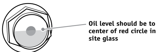
Figure 3: Check proper oil level
