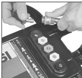
**⚠ WARNING** **Risk Of Injury. Ensure nozzle is completely inserted in QC socket, and QC snap ring is fully engaged (forward) before squeezing gun trigger.**
