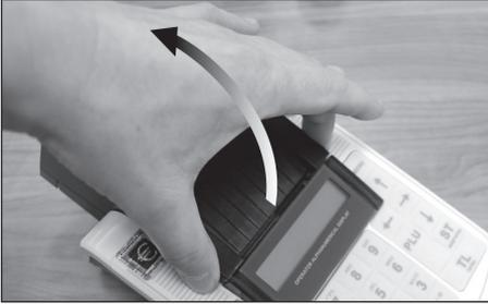
2. Press the printer roller release lever to release the printer roller, and then lift it.
