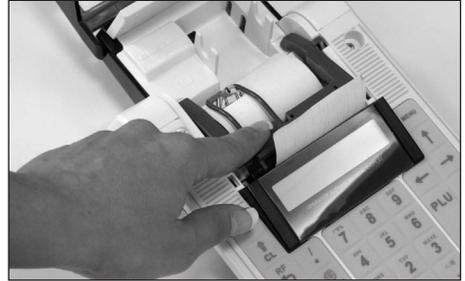
5. Press the paper-feed button (4) to be sure the roll properly advances.
