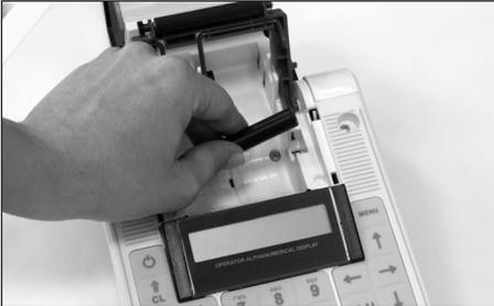
4 Hold the ends of the ribbons upended through the display and return the printer roller (3) to the
