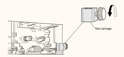
4. Insert the blade holder into the hole in the carriage.
