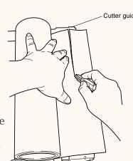
3. Insert the media in the machine's feed unit. Insert the media until it makes contact.
