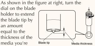
Turn clockwise to extend the blade. Turn counterclockwise to retract the blade. The blade is extended by 0.0196 in. (0.5 mm) with
