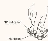
4. Arrange the ink cartridges so that side B faces up and grasp the ink cartridge at the center using your thumb and index
