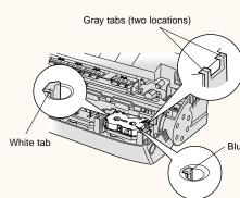
6. Make sure the ink-ribbon cartridge is held securely by the white tab, blue tab, and two gray tabs on the inkribbon cartridge holder, and that there is no slack in the Blue tab ribbon.
