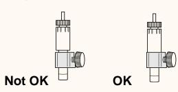
5. Turn the tool-carriage screw clockwise to secure in place.
