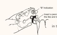
2. As shown in the figure, insert a pencil or the like into Insert a pencil or side B of the ink-ribbon the like and turn. cartridge and turn clockwise to take up slack in the ink ribbon.
