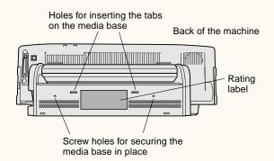
With the roller side of the media base facing up, insert the tabs on the media base into the holes on the machine.
