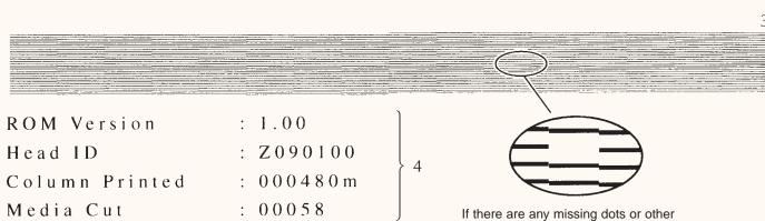
evidence of a drop in printing quality, clean the head. For more information about head cleaning, see 6-1 in the User's Manual: "Cleaning the Printing Heads."
