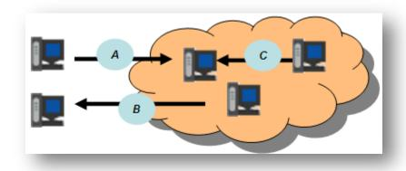
In the above picture, three sessions labeled A, B, and C are shown communicating to, from, and inside a focus network. In session A, the PVS only analyzes vulnerabilities observed on the server inside the focus network and does not report client side vulnerabilities. In session B, the PVS ignores vulnerabilities on the destination server, but reports client side vulnerabilities. In session C, both client and server vulnerabilities are reported.
