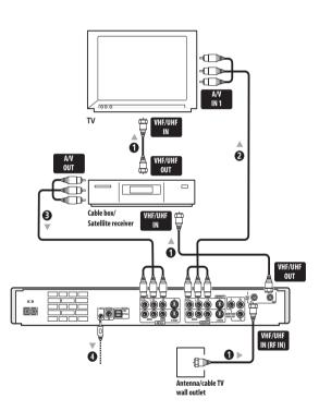
Connect RF antenna cables as shown.
