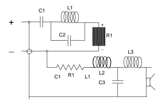
Note: If additional low frequency output is desired for your application an additional 10 watt-8 ohm resistor can be placed in parallel with R1. This resistor is located on the back of the woofer. Contact the factory for the resistor or if you have any questions regarding this.
