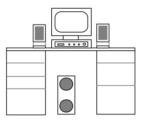
Make the electrical connections to the speakers as shown on the next page. Plug in the right desktop speaker cable (1/4 inch phone plug) into the socket on the back of the woofer cabinet designated "right" and the left desktop speakers cable into the left socket. The cable coming from the amplifier speaker output terminals is attached to the center connector.
