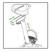
upward or downward to the desired position, and then release the knob. Move the seat post upward or downward slightly to make sure that the knob is engaged in one of the adjustment holes in the seat post. Then, tighten the knob.
