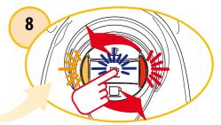
The long espresso button and the descale and alarm indicator lights blink alternately. Press the long espresso button to start the descale cycle.
