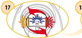
At the end of a rinse cycle, the long espresso button and the descale and alarm indicator lights blink alternately and the machine beeps.
