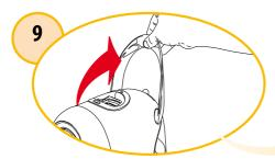
Raise lever to eject used capsule into the used capsule container.
