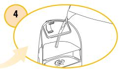
Prepare the descaling solution following the manufacturer's directions and pour a liter of solution into the tank.
