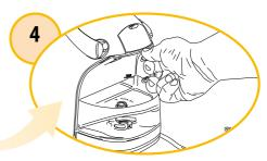
Remove the water tank. Empty and rinse. NOTE: The water tank is NOT dishwasher safe.
