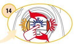
The long espresso button and the descale and alarm indicator lights blink alternately. Press the long espresso button to start the rinse cycle.
