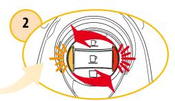
When the descale and alarm indicator lights blink alternately and the machine beeps, it is necessary to carry out a descaling cycle.
