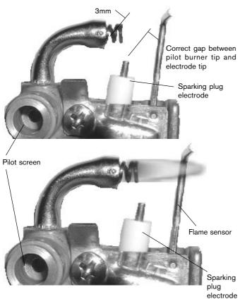
Fig. 12 - Characteristic Pilot Flame
