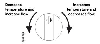
Figure 11 - Principles of Operation
