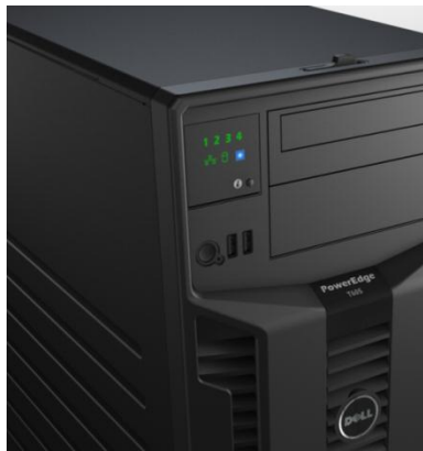
Figure 5. LED Control Panel
