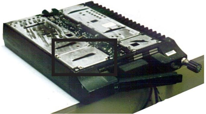
Refer to the audio squelch board layout for the location of JU201. If JU201 is not installed, add this jumper using a short length of insulated wire. This finishes work with the audio squelch board. When you place this board back in the radio, be sure that the 6 pins that plug into the audio power amplifier board (2 transistors on a heatsink mounted to the side of the radio) mate correctly.
