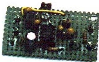
Picture of Perf Board for TAPR/G3RUH Buffer Amplifier.
