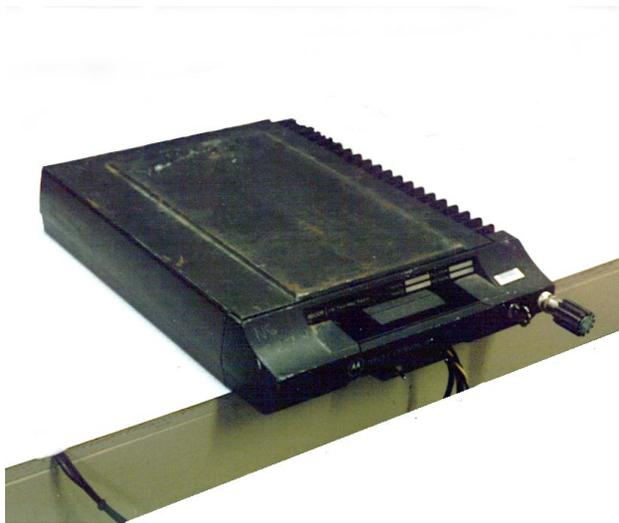
The transmitter employs a heterodyne exciter. Receiver oscillator injection is mixed with the signal from an offset oscillator to generate the transmit frequency. The offset oscillator is varactor modulated for true FM.
