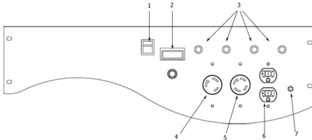
**Engine Switch (1)** – Flip the switch to the “On” position and pull the recoil starter to start the generator. Turn to the “Off” position to turn off the generator.
