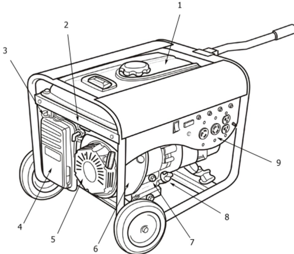
**Fuel Tank (1)** – 6.5 gallon capacity fuel tank.
