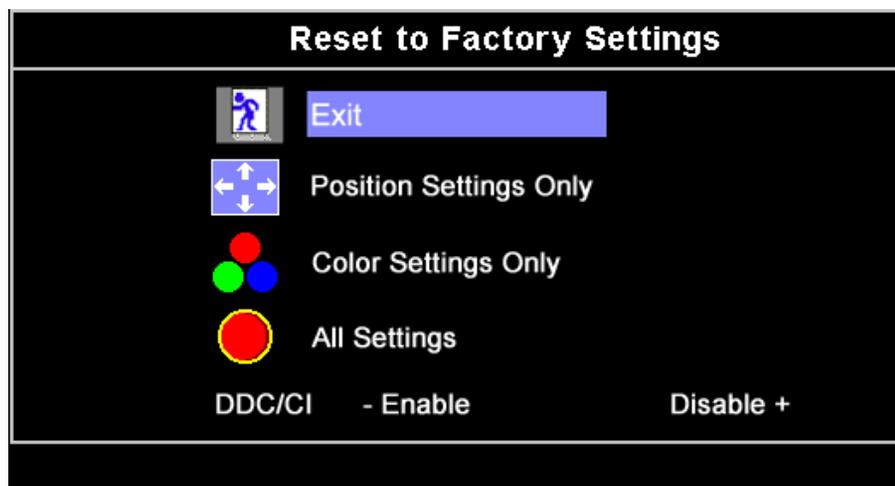
**Exit** — Select to exit out of Reset to Factory Settings menu without resetting any OSD options.
