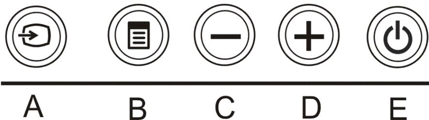
Use the Input Select button to select between two different video signals that may be connected to your monitor.
