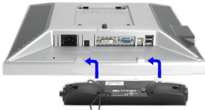
1. Working from the rear of the monitor, attach the Sound Bar aligning the two slots with the two tabs along the bottom rear of the monitor.
