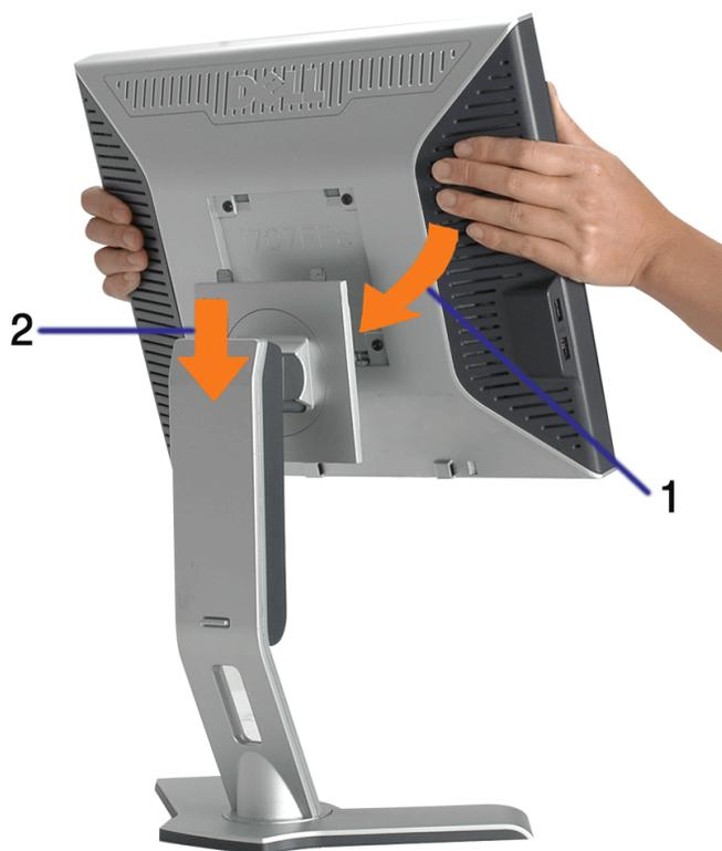
1. Fit the groove on the monitor to the two tabs on the stand.
