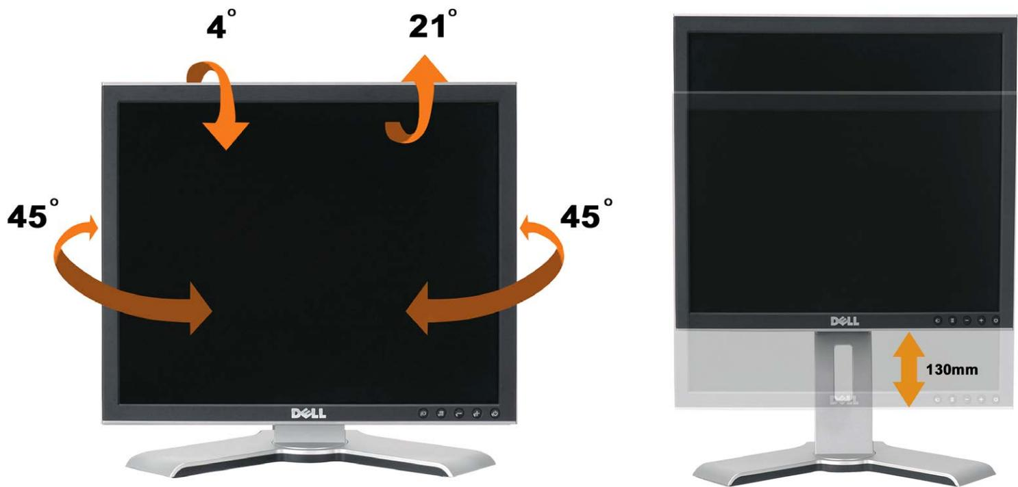
You can adjust the stand vertically, up to 5.12 inches (130mm) using the stand lock/release button. You can adjust the monitor to the desired position by sliding the monitor up and down the Stand. .
