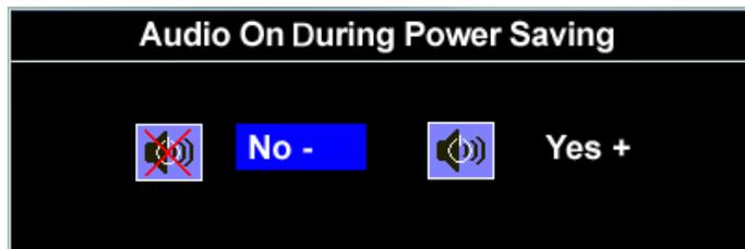
**NOTE:** When the Dell Soundbar is not properly connected to the monitor, the audio menu is not available.
