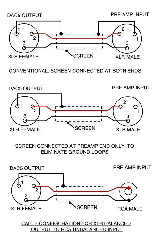
When connecting the XLR / BALANCED outputs to a pre amplifier with an RCA / Single Ended input, the switch must be set to the 'SINGLE ENDED' position.
