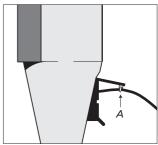
For safety reasons you must fasten the mains lead to the black lid using the enclosed cable-tier (A).
