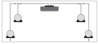
The special adaptor, part no. 6270706, can be used to connect additional pairs of loudspeakers to your Bang & Olufsen system. The adaptor is available as an optional accessory from your Bang & Olufsen retailer.
