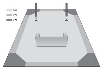
Position zones: The three settings (free, wall and corner) correspond to the position zones marked in different shades of grey.
