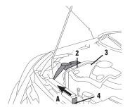
**Screen washer fluid level** Add some fluid to reservoir **2** if necessary.
