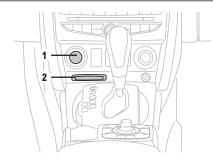
**Stopping the engine**With the vehicle stationary, press button 1.
