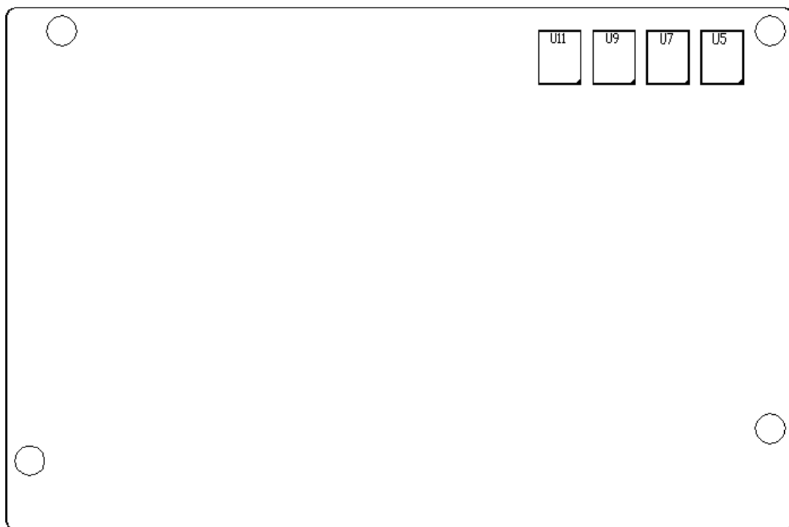
Figure 2.3: Jumpers and Connectors Location- Board Bottom
