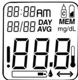
The test strip and flashing blood drop tells you the meter is ready for you to apply a drop of blood to the sample application tip at the end of the test strip.
