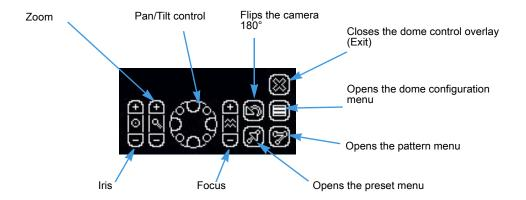
Center buttons allow automatic control: auto iris, auto zoom, and auto focus. The center of the Pan/Tilt Control stops camera movement.
