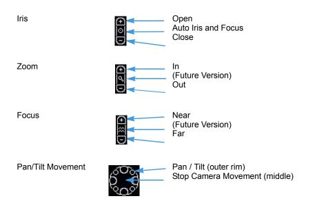
These camera handlers enable access to these dome configuration menus:
