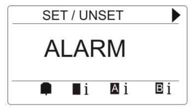
Press the softkey below the blinking alarm symbol.
