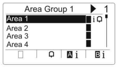
4. Press the softkey below the blinking alarm symbol.
