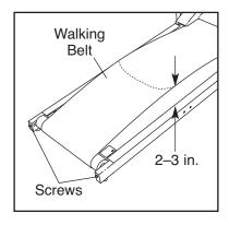
ment screws counterclockwise 1/4 of a turn. When the walking belt is properly tightened, you should be able to lift each edge of the walking belt 2 to 3 in. (5 to 7 cm) off the walking platform. Be careful to keep the walking belt centered. Walk on the treadmill for a few minutes. Repeat until the walking belt is properly tightened.
