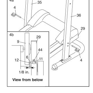
Hold the Handrail (5) near the Left and Right Uprights (35, 36). Connect the Handrail Wire (2) to the Reed Switch Wire (6). Insert the Wires down into the Left Upright.
