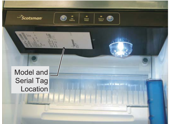
Control Panel, Bin Light and Curtain
