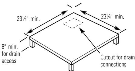
The ZVAC requires a field supplied installation platform. The installation platform must be a minimum of 23 1/4" square, with legs to raise the platform a minimum of 8" (12"
