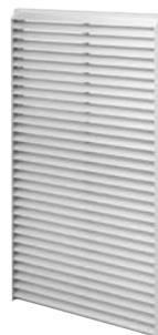
The architectural louver exterior grille is mounted to the exterior flange of the plenum and held in place with four screws inserted from inside enclosure closet. The grille is designed specifically for use with the ZVAC unit and the use of any other grille must be approved by GE Air Conditioning Applications Engineering.
