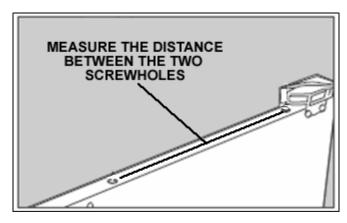
**5)** Measure the distance between the two screw holes on the top of the freezer door.
