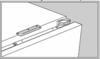
**12)** The bracket at the top of the freezer door should be flush with the underside of the work top.
