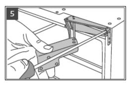
**5)** With the top hinge open, undo the screws holding it to the cabinet and then remove it.
