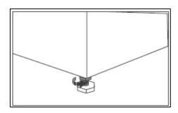
Fully tighten the locking nut on each leg, against the underneath of the freezer.
