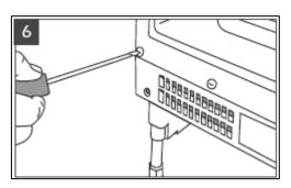
**6)** Remove the blanking plates for the cabinet
