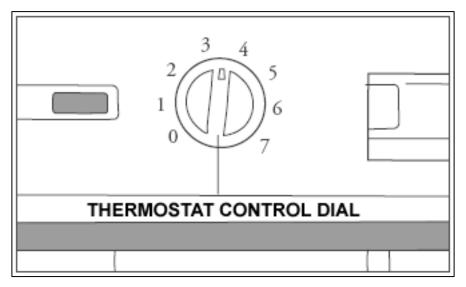
You switch on your appliance by connecting it to your mains supply and setting the thermostat. The thermostat control knob is located at the bottom of the appliance, near to the ventilation grill.
