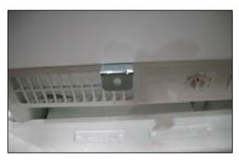
10) At the bottom of the freezer door, there are two holes. You should secure the lower fixing brackets to these holes using the screws provided. The longer section of the lower fixing bracket should be connected to the bottom of the freezer door.
