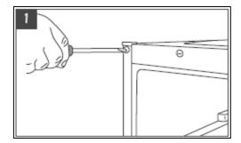
**1)** Remove the blanking plates from the outside of the appliance door.
