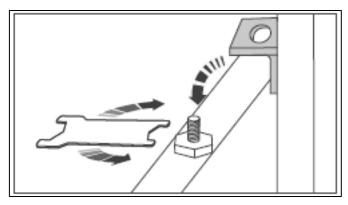
**9)** Tighten the upper retaining bolts to the top of the appliance door.
