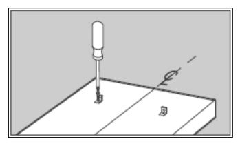
**8)** Using the screws provided, secure the front brackets to the inside of the furniture door on the holes that you have just drilled.
