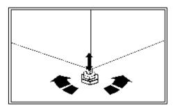
o Turn the foot to either raise or lower the height of the freezer.
