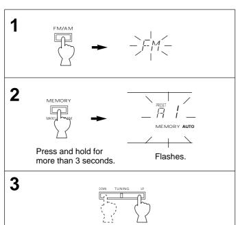
To tune to higher frequencies, press right side once. To tune to lower frequencies, press left side once.
