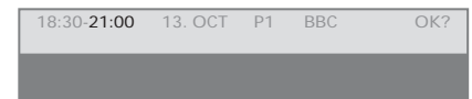
The status line for a recording may appear above the teletext page with both start and stop times indicated, or on the actual program you want to record.
