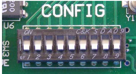
Figure 7.1 SW 3 (CONFIG Switch bank)
