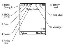
Signal Strength Indicator – Vertical bars show the strength of the network connection. You can't make or receive calls when T or TO shows. 2 EDGE/GPRS Indicator – Shows when your phone is using a high-speed Enhanced Data for GSM Evolution (EDGE) or General Packet Radio Service (GPRS) network connection. Indicators can include:
