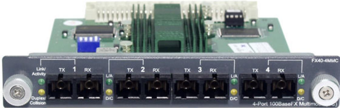
When installed into a switch, this module provides 4 x 100 Mbps Fast Ethernet fiber ports that can be used to connect the switch to the network backbone, a 100 Mbps server or end station.
