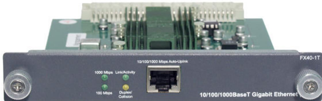
When installed into a switch, the FX40-1T Gigabit module provides one Gigabit Ethernet port that can connect the switch to a Gigabit backbone switch or to a server with a Gigabit NIC adapter card.
