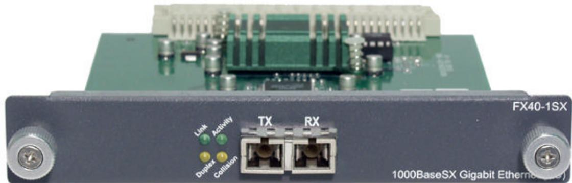
When installed into a switch, the FX40-1SX (50, 62.5/125 micron multi mode fiber optics to 2 Km) and the FX40-1LX (8,9/125 micron single mode fiber optics to 60 Km) modules each provide one Gigabit Ethernet port that can connect the switch to a Gigabit backbone switch or to a server with a Gigabit NIC adapter card.
