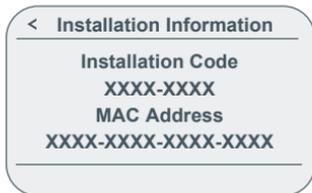
**STEP 3** Once you have provided the two numbers above you will be asked to send a “Join” request from the thermostat. To do so go to the NETWORK CONNECTION screen.
