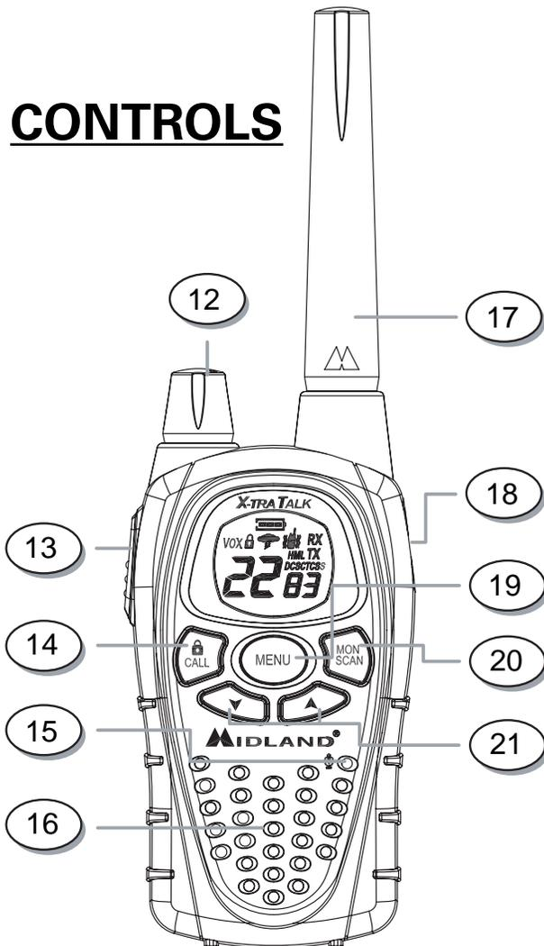
12. **POWER/VOLUME KNOB** – Turn clockwise to turn the power on and increase the volume level. Turn counter-clockwise to decrease the volume level and turn the power off.
