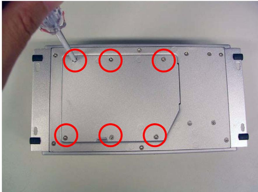
**Figure 2.11 Unscrew the HDD door screws**
