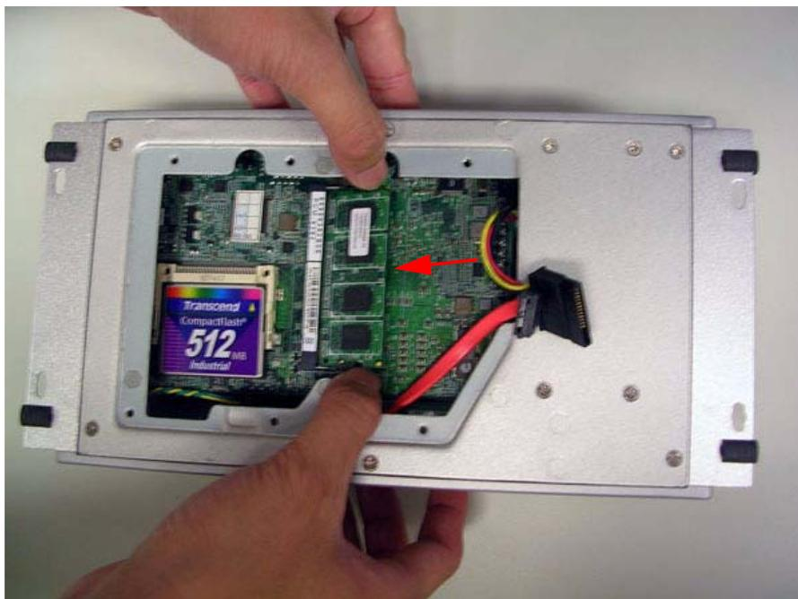
**Figure 2.15 Install the memory module into the SO-DIMM socket at the bottom of the Main board**
