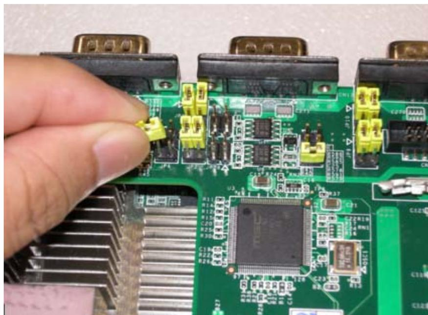
Figure 2.17 RS-232/422/485 jumper setting
