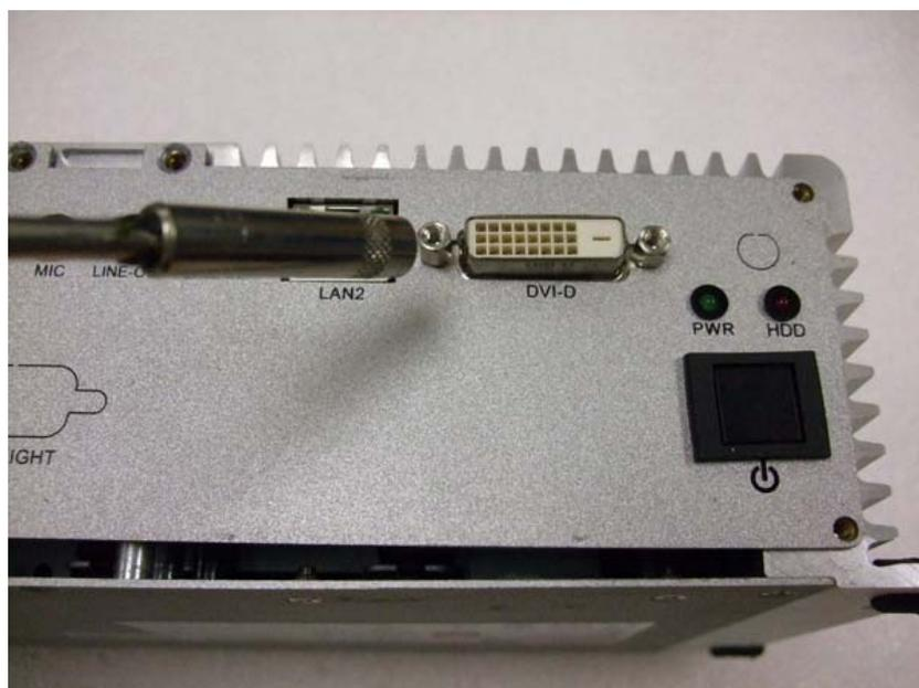
**Figure 4.4 Unscrew the hex-bolts on the panel**
