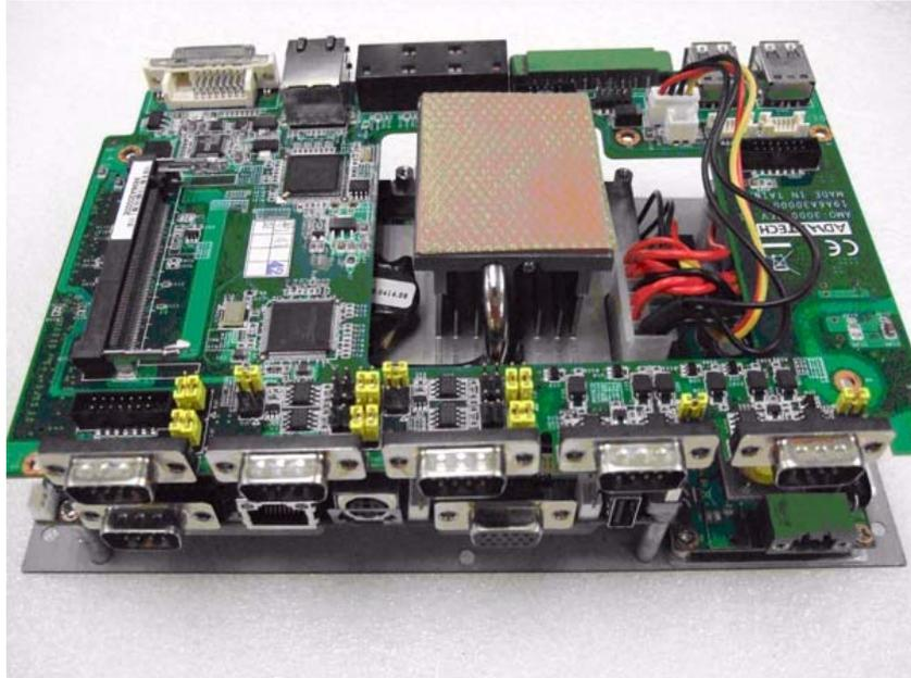
**Figure 4.5 Unscrew the screw fixed AMO-3000 on MB**
