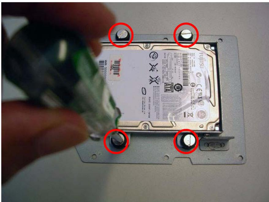
Figure 2.13 Screw on the HDD damper screws to assemble the HDD door and HDD frame
