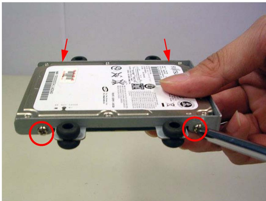
Figure 2.12 Assemble HDD and HDD frame by 4 Screws
