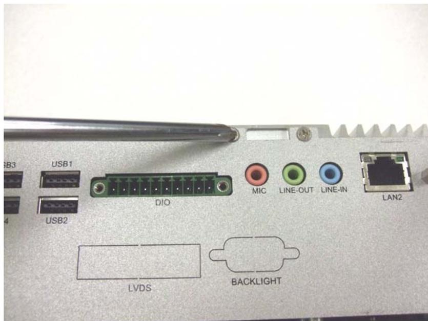
**Figure 4.3 Unscrew the panel screws**
