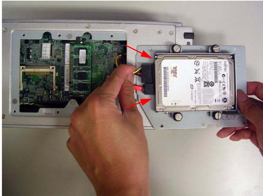
**Figure 2.14 Connect the HDD cables**
