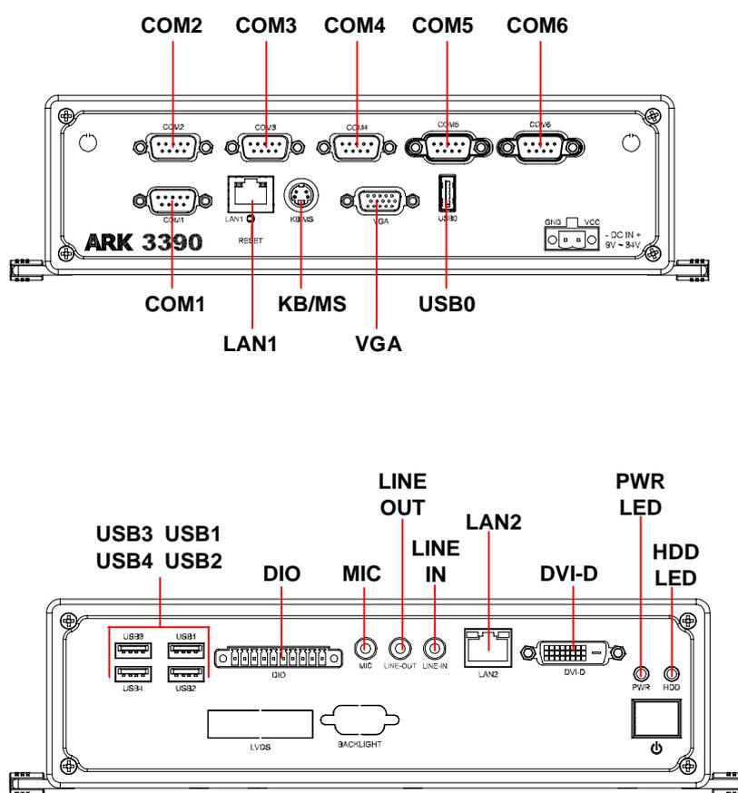
Figure 2.1 ARK-3389 IO connectors drawing
