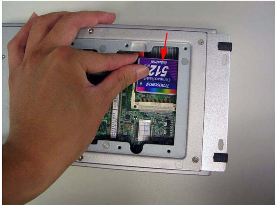
Figure 2.16 Install the CF card into the CF slot at the bottom of the Main board
