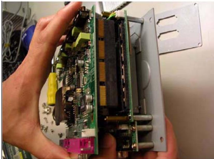
**Figure 4.6 Remove AMO-3000 from MIO socket of the system board**
