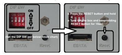
DIP switch code(from left to right) "DIP switch 1", "DIP switch 2" and "DIP switch 3" "DIP switch 4".
