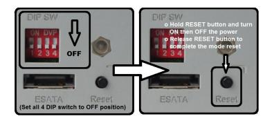
B. To set the DIP switch to a new RAID mode, please follow the mode chart as below, press the RESET button and hold it, turn on the box and keep hold reset button for 15sec.
