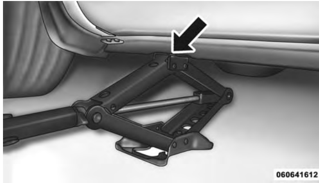
Front Jacking Location
