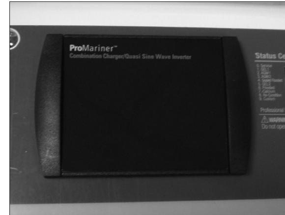
1) Locate remote panel and prepare an appropriately sized mounting location (75mm x 44mm or 3" x 1-3/4"). A connector and extension cable are provided. The extension cable is to be connected to the external connection as indicated in the FEATURES section.
