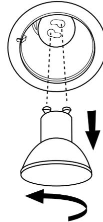
3. Remove the bulb and replace it with a 120-volt, 50-watt maximum halogen bulb with a GU10 base. Turn it clockwise to lock it into place.
