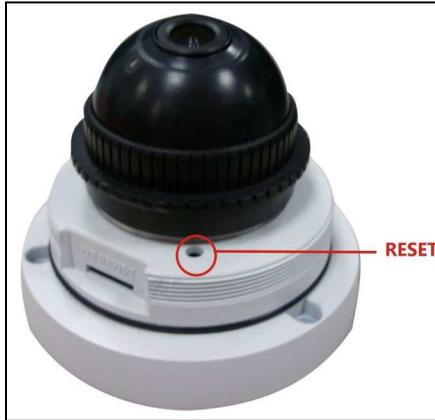
3. Press and hold the button and connect power and Ethernet cable to the camera again and hold for round 20 seconds for system booting.
