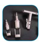
The En Core® Sampler, a disposable volumetric sampling device, was developed to assist field personnel in taking soil samples with minimal handling and maximum accuracy.
