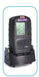
The typical confined space monitor measures oxygen, combustibles, carbon monoxide, and hydrogen sulfide.
