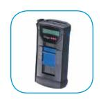
CMS does not require gas calibration. All measurement and calibration information is stored on a bar code on the CMS Chip. An electronics and leak check is performed before each measurement so you are assured of accurate indications every time. Operating on 4 "AA" cells, the CMS will deliver about 100 measurements per battery change. Popular applications include TWA screening, confined space entry, and emergency response.
