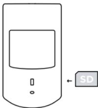
**IMPORTANT NOTICE: The PIR-SD required an SD card to be inserted into the SD slot in order for the PIR-SD to function as a motion detector/recorder.**
