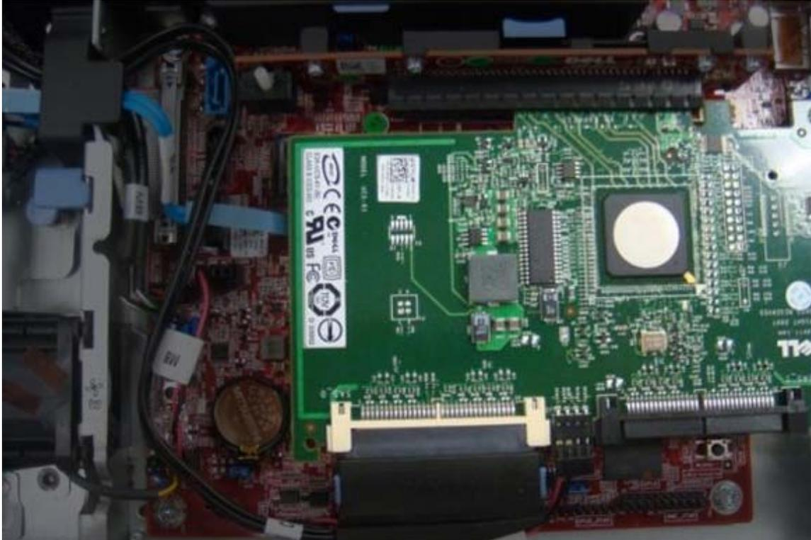
**Figure 14.** SAS 6/iR Adapter Card Installed
