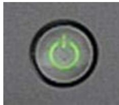
**Figure 4.** Power Button LED
