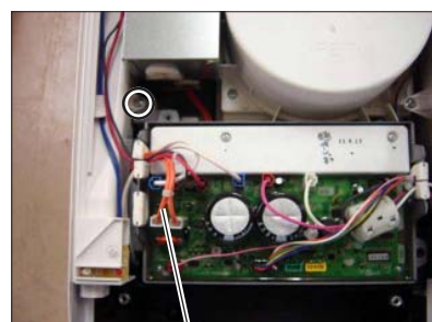
Filter circuit board lead wires (orange)
