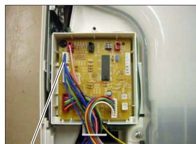
Display circuit board lead wires (blue)
