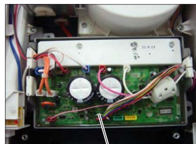
Power circuit board (JT-30P3H/JT-30P3)
