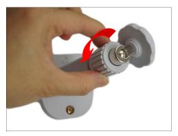
3. Screw the camera to the bracket.
