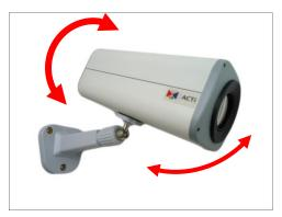
6. Tighten the knurled knob to fix the camera position.
