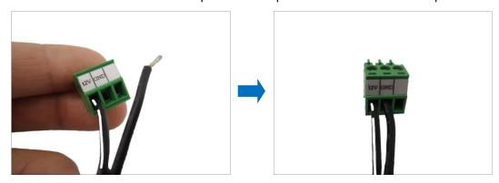
4. Tighten the screws of the 12V pin and the GND pins to secure the wire connection.
