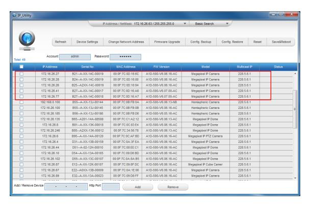
You can quickly notice the camera model in the list. Click on the IP address to automatically launch the default browser of the PC with the IP address of the target camera filled in the address bar of the browser already.
