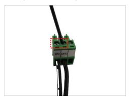
5. Set the prepared power adapter for connection later. Below is an example of a power adapter with an attached terminal block.
